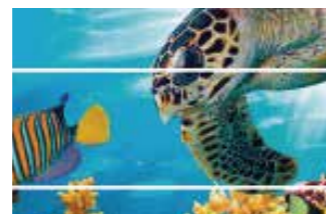
Gap/White streaks (Excessive feeding amount)
