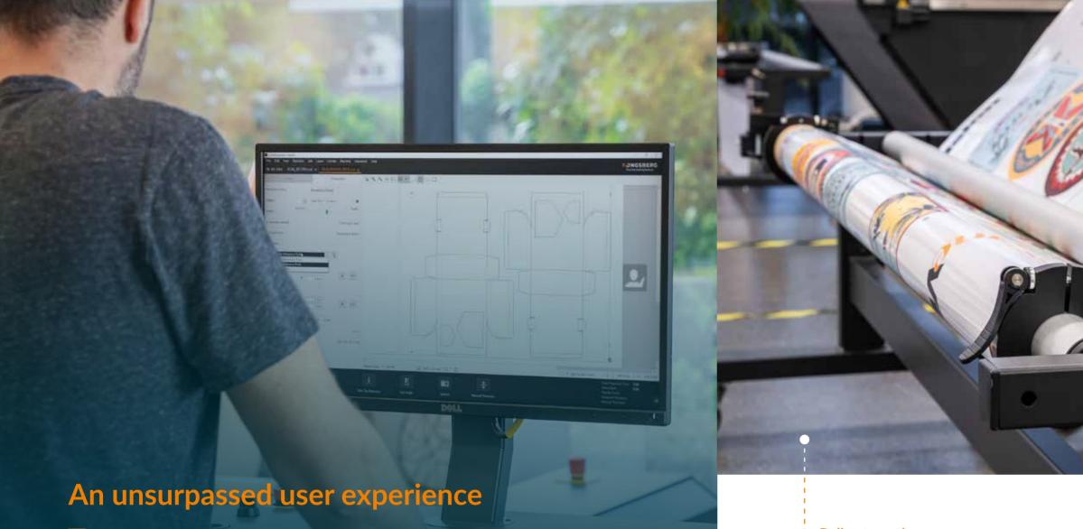
The i-cut Production Console, the front-end for the Kongsberg X, works with a graphical icon-based communication which allows the operator to supervise production from a distance. A separate operator login ensures personalized language settings and job list management.
